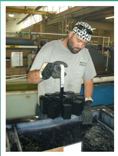
One PAS II~III@ Pending and all work on that bar anodizes at the same ASF
