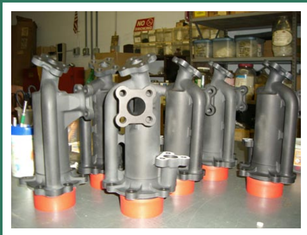
Intricate castings done using ASF
